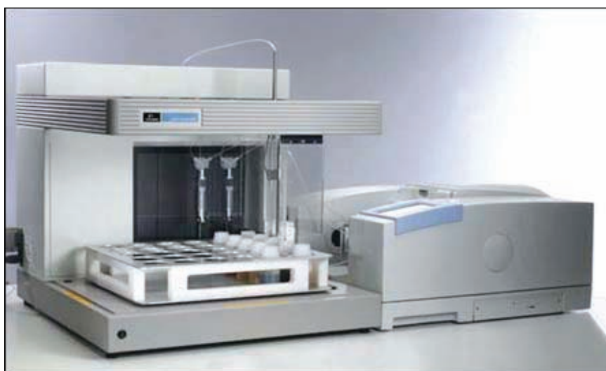
Figure 1 Typical instrumentation for determination of FAME in middle distillates
