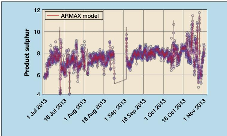
Figure 4 Predicted vs actual diesel sulphur content
