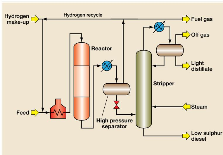
Figure 1 Diesel hydrotreating unit schematic
