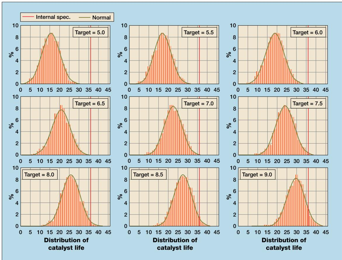
Figure 11 Catalyst life distribution – reactor dP limited
