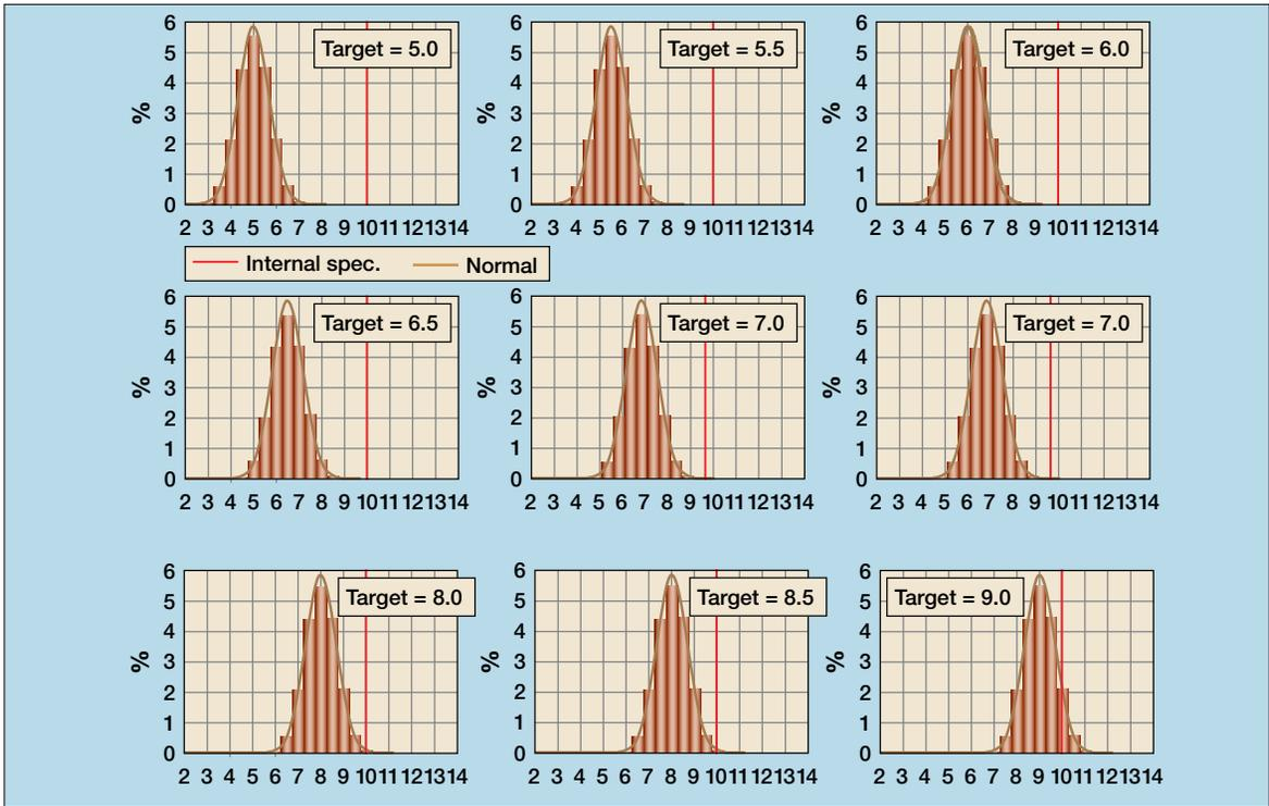
Figure 8 Sulphur distribution – one-hour data
