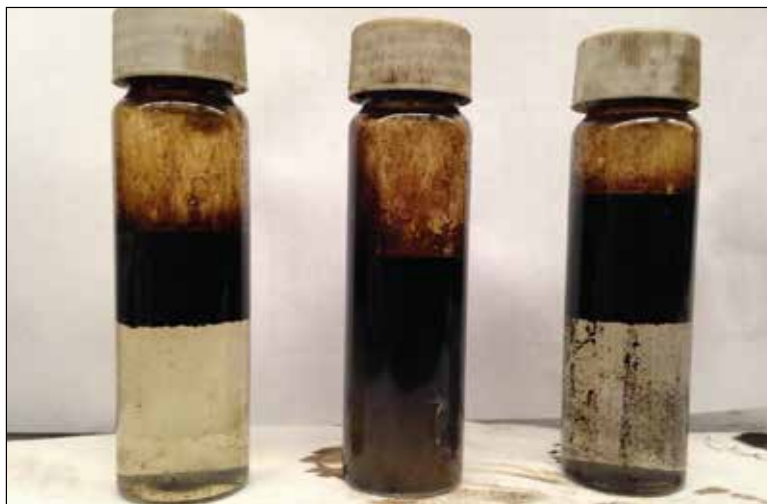
Figure 5 From left to right: an emulsion treated with caustic, no chemistry, and a standard emulsion breaker
